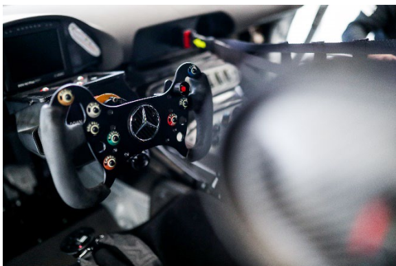
The Mercedes-AMG GT3 manages entirely without a mechanical connection between the steering unit and the steering gear. The steer-by-wire system from Schaeffler Paravan makes this possible and is also an important key technology for autonomous driving. Photo: Group C Photography
